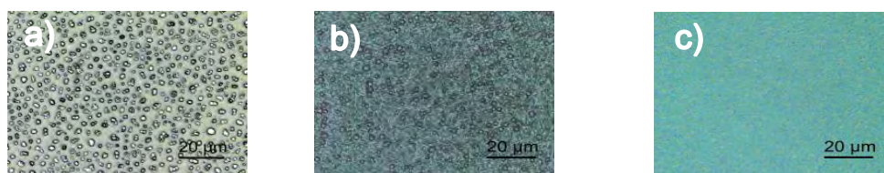
Fig. 1: Laser scanning microscopy: CuI deposition by a) CVD on a PLD CuI buffer layer (CuI islands), b) Bädeker route: Cu deposition at 310 °C and iodization at room temperature (CuI layer), c) Bädeker route: Cu deposition at 210 °C and iodization at room temperature (CuI layer).
